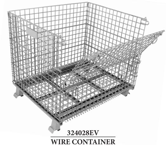
The side and base mesh is  $2" \times 2"$  ( $5 \times 5$  cm). The gate is a 1/2 drop front gate with only four latch bolts to engage for quick and easy assembly. The 324028 has four way entry for forklifts or pallet jacks, with a clearance of 4.5" (11.4 cm). Can be stacked up to four high fully loaded. The casters are  $4" \times 2"$  Phenolic, 2 Rigid and 2 Swivel.
